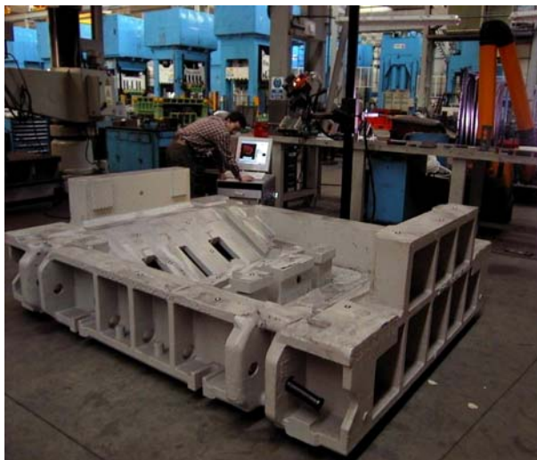
复杂铸件模具的质量检测: 3000 \times 2000 \times 1000 \text{ mm}^3
