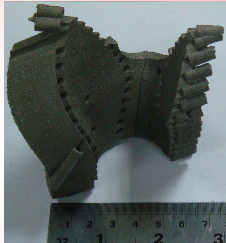
Stainless steel guide-1 manufactured by SLM
