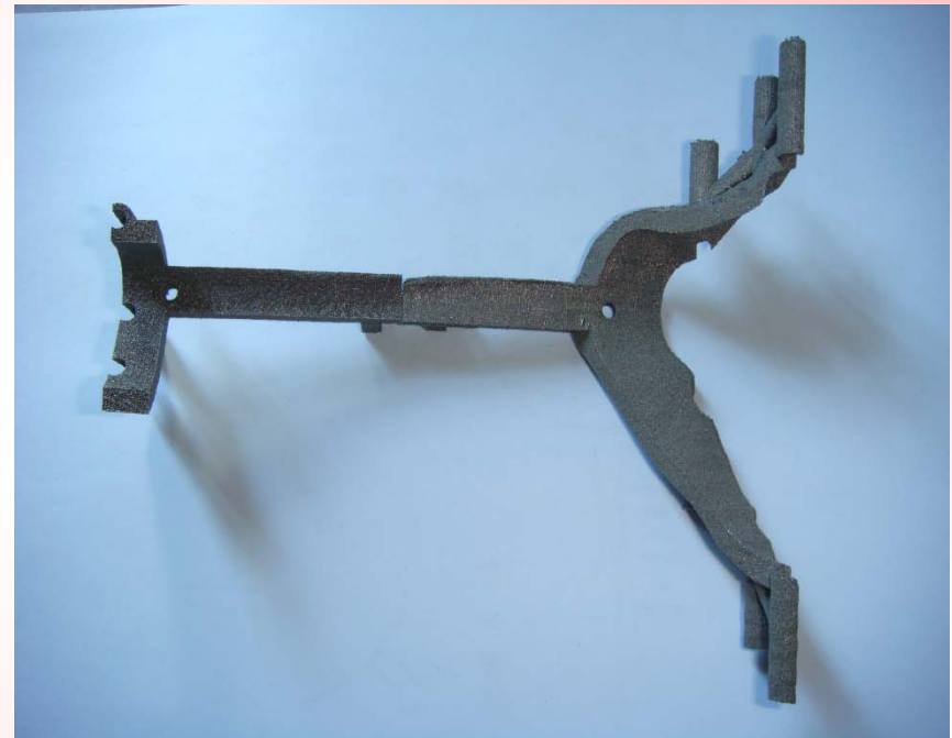
Stainless steel guide-2 manufactured by SLM
