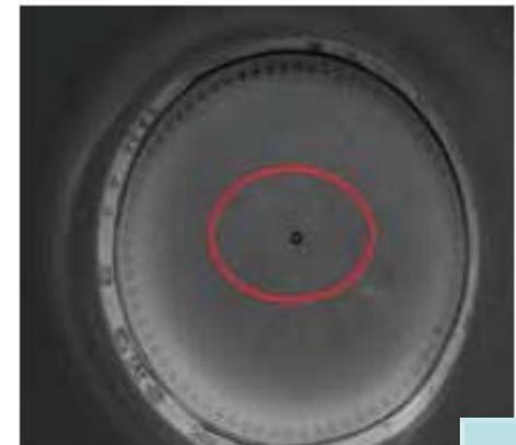
瓶底气泡 | Bubble on the bottle bottom
