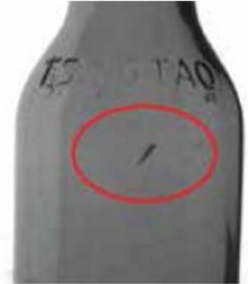
短裂纹 | short crack
