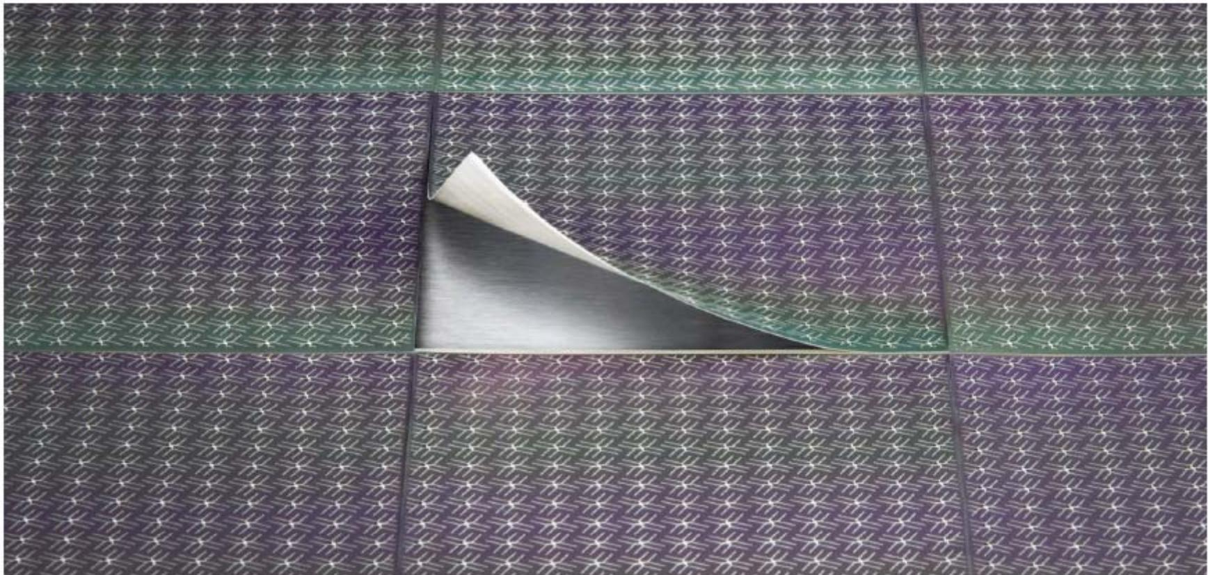
**Figure 15:** Nanosolar MWT back-contact cells are interconnected into electrical circuits via tabs on each cell that are simply the overhang of one of the two laminated aluminum foils. Dr. Mike McGehee, Stanford university
