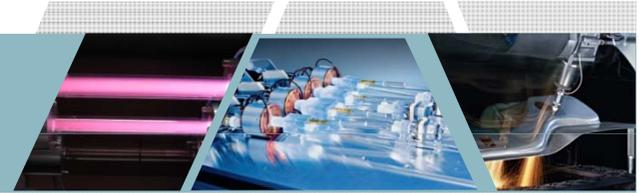
**The 2 kW DIO CUT system can be applied in oxygen cutting. The cutting edge quality is comparable and the speed is very close to the speed of fiber and CO<sub>2</sub> lasers.**
