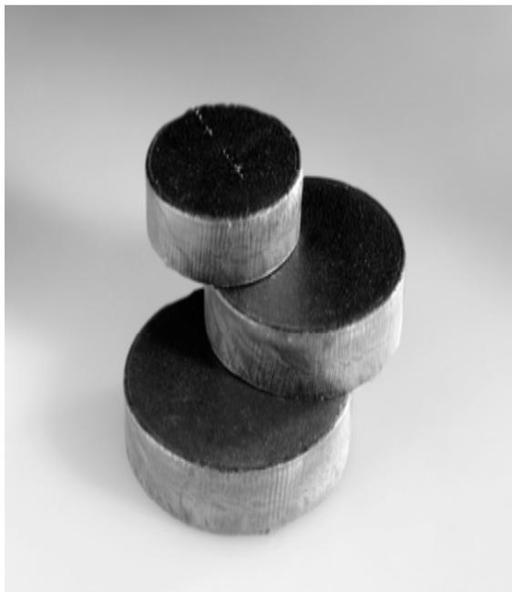
**Autogenous contour cuts in 10mm mild steel ( $v=0.45$  m/min, nozzle:FK4 60-100)**
