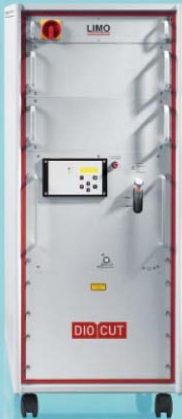
The “DIOCUT” system enter the laser macro cutting market. The system is demonstrated by cutting aluminum, stainless steel, copper and mild steel. The cutting edge quality is comparable with CO2 laser cuts.
