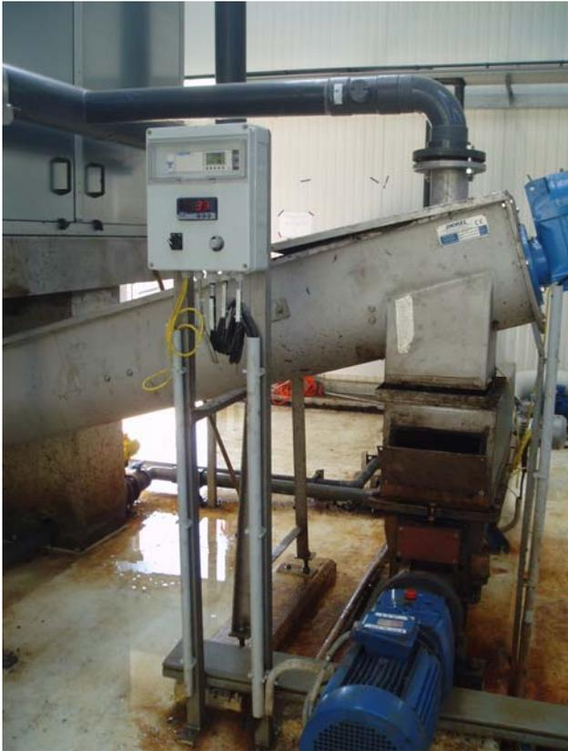
Screw conveyor to feed to the GBB
