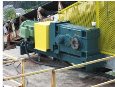
Aggregate Quarry 210K MagnaGear with Backstop & Swingbase
