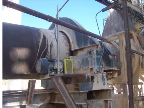
Limestone Dryer 285K MagnaGear w/60Hp motor
