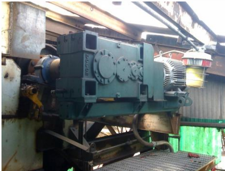
Coal mine refuse belt 150K MagnaGear w/75 Hp motor & swingbase
