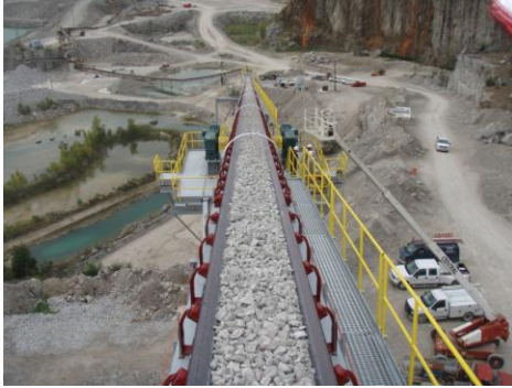
Aggregate Quarry 2 – 525k MagnaGear w/300 Hp motors
