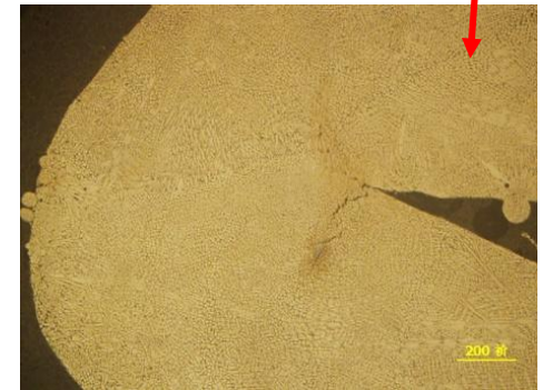
Micro cracks at TE
