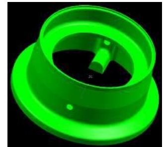
Flame Check Valve Flange
