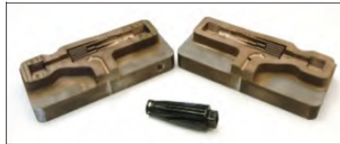
Tooling inserts made with direct metal laser sintering from EOS, courtesy of Morris Technologies
