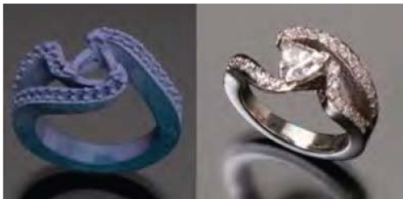
Wax pattern (left) made on a machine from Solidscape and final product (right), courtesy of Caitlin Skelcey
