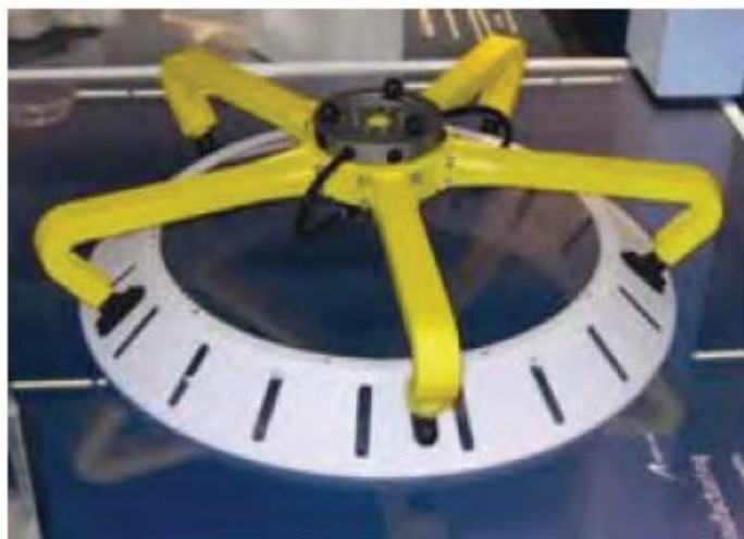
Robotic vacuum gripper made by FDM, courtesy of Digital Mechanics AB
