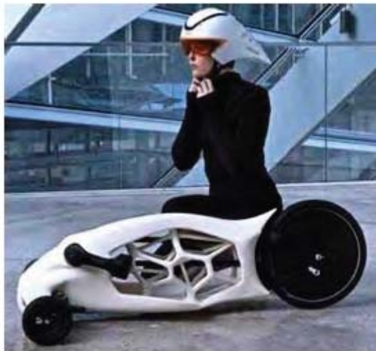
Hand drill-powered vehicle made by FDM, courtesy of HAWK-University of Applied Sciences and Arts
