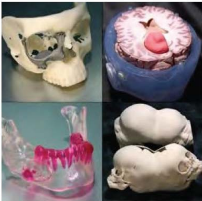
Medical models produced by AM, courtesy of Medical Modeling Inc.
