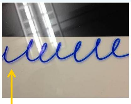
Poor permanent marker ink repellency on freshly cured **COMP3**
