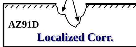
Fig. Schematic of the corrosion progress on JDBM and AZ91D
