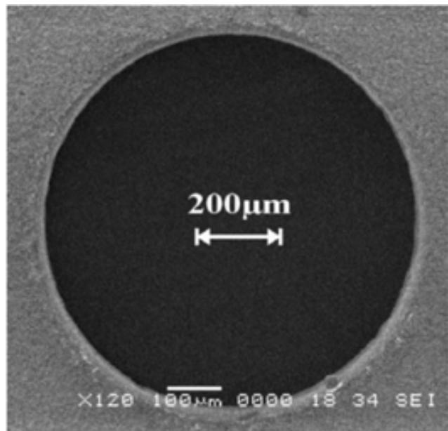
1 mm hole drilled in a 200  $\mu\text{m}$  thick ceramic sheet
