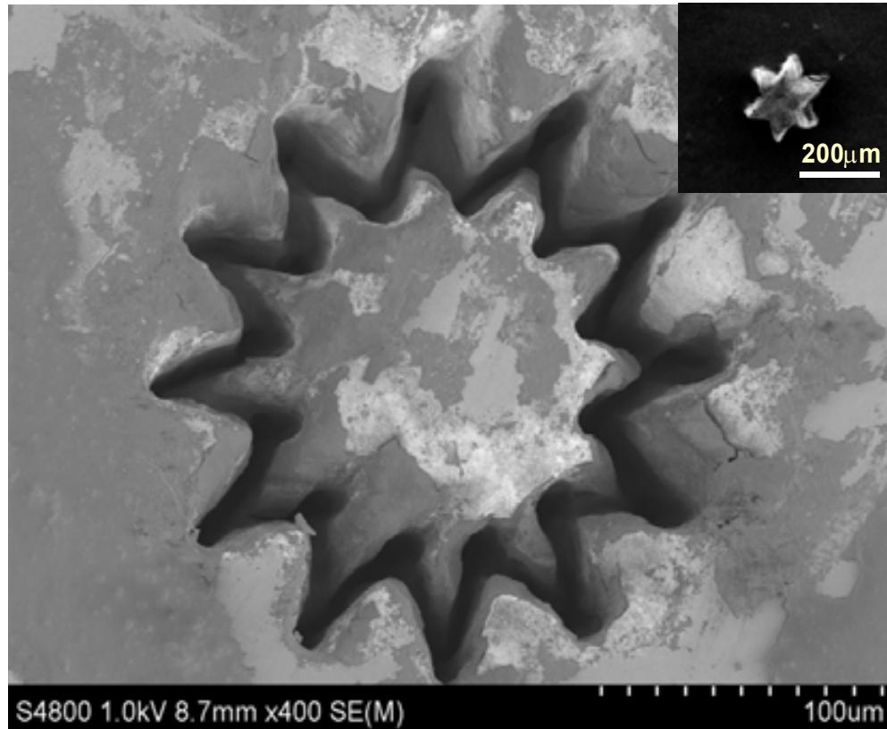
SiC microgears cut by fs laser
