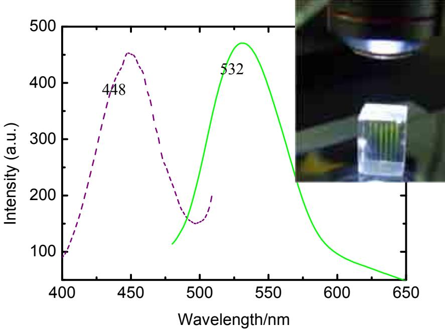
Emission and excitation spectra for the fs laser-induced color centers in LiF
