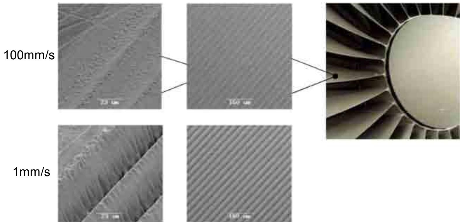
Riplet structures on metallic surfaces with reduced friction
