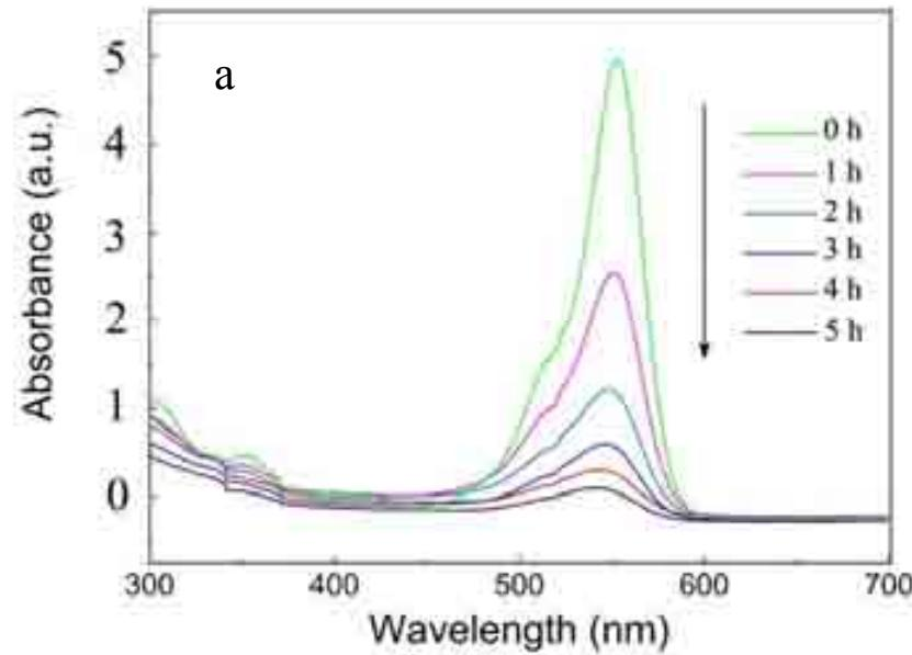
Absorption spectra of RB solution catalyzed by the ZnO nanostructure under UV irradiation.
