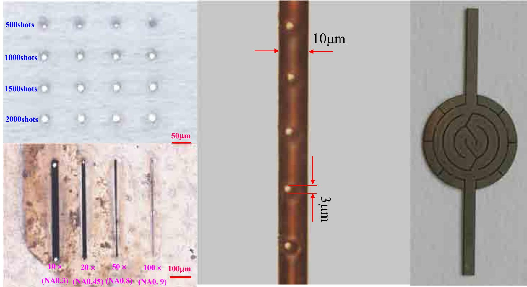
Drilling and cutting of tungsten by fs laser
