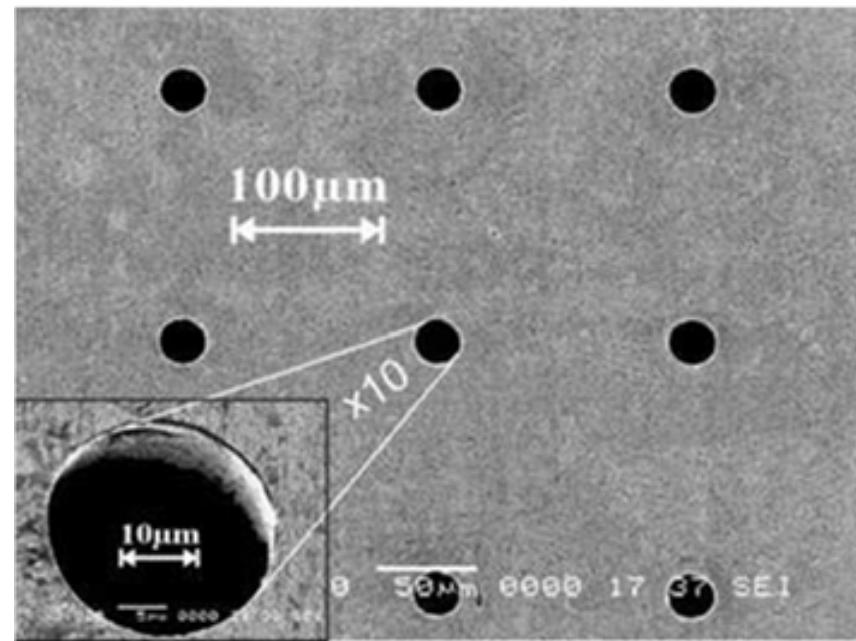
$30 \mu\text{m}$  diameter hole drilled in  $25 \mu\text{m}$  steel foil
