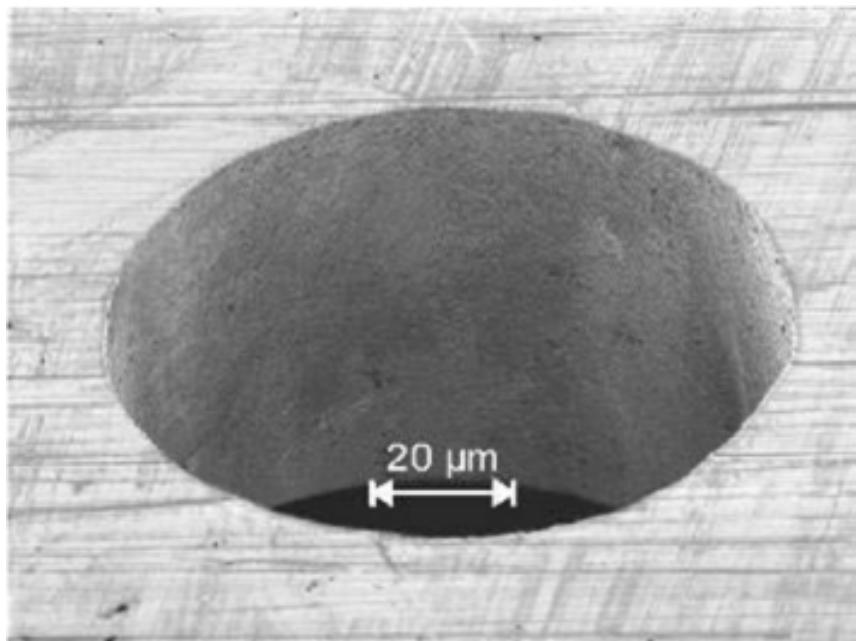
Hole ( $\phi 100 \mu\text{m}$ ) drilling in  $100 \mu\text{m}$  steel sheet
