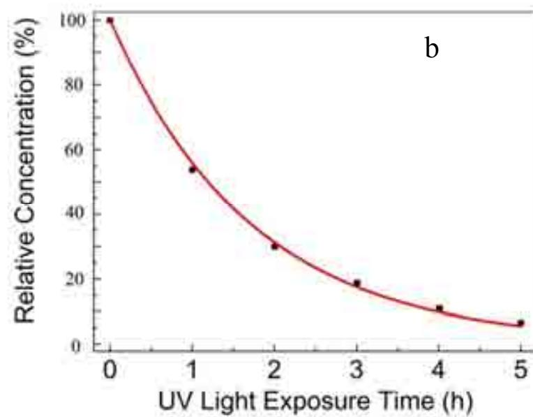
Degradation of the RB under UV irradiation as a function of time.
