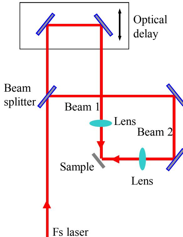
Precise adjustments of optical delay by observing the SHG or THG to obtain the temporal overlap of femtosecond pulses.
