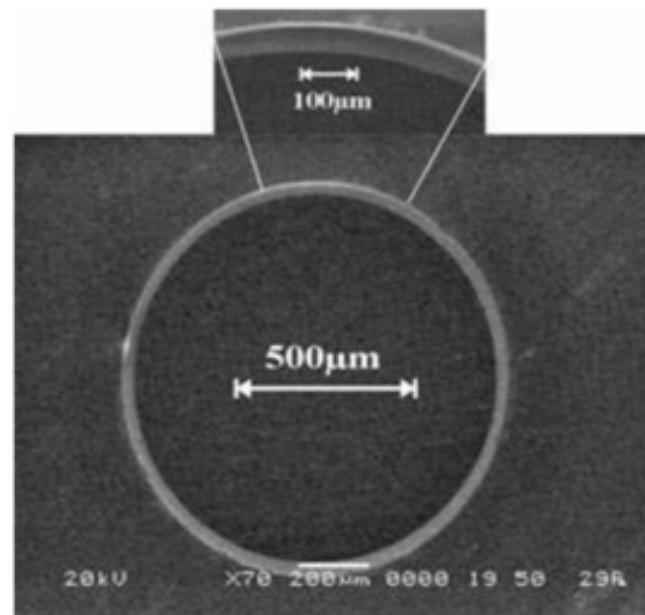
1 mm hole drilled in a 140  $\mu\text{m}$  thick glass coverslip
