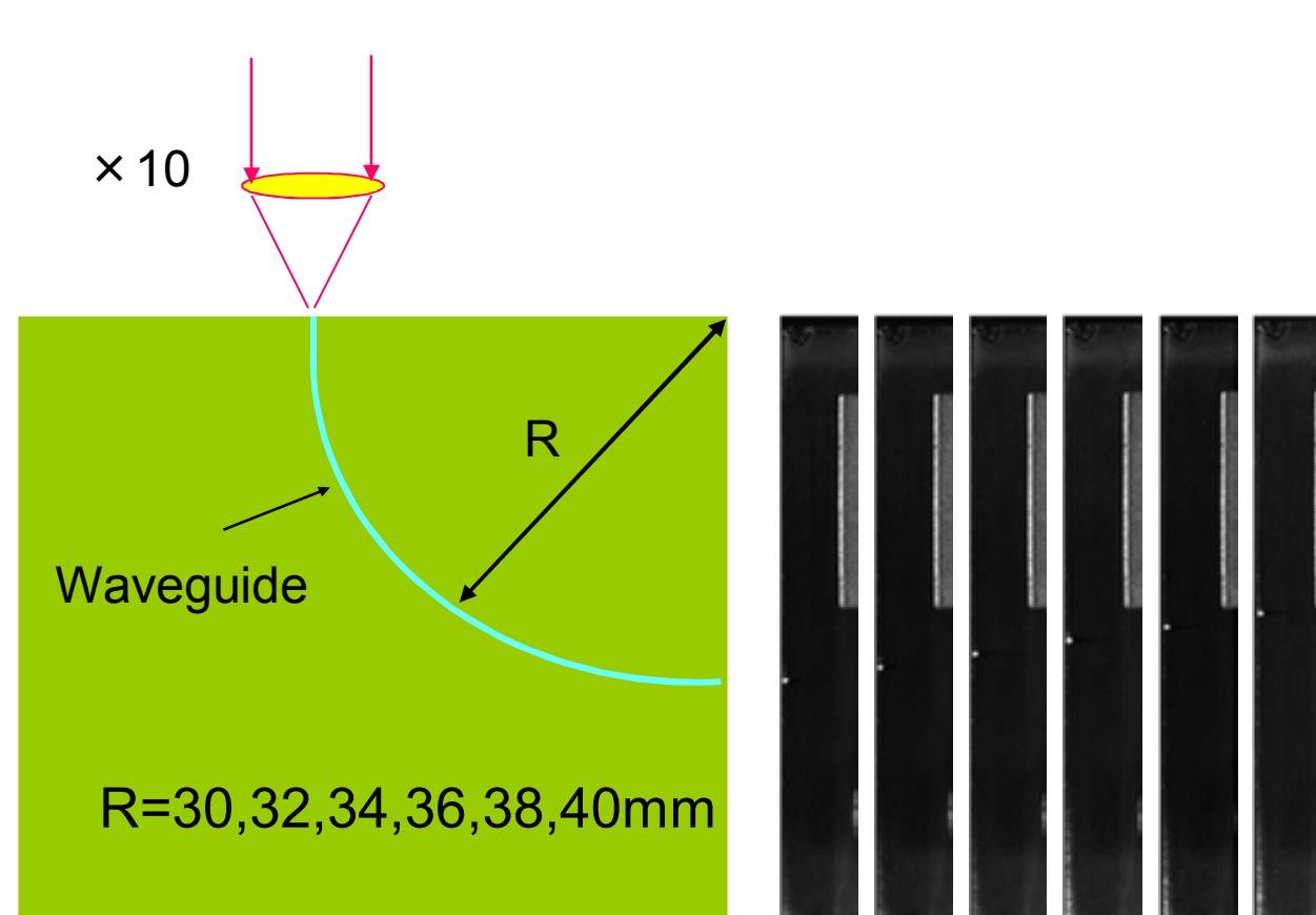
Transmission light of the end face of bending waveguides
