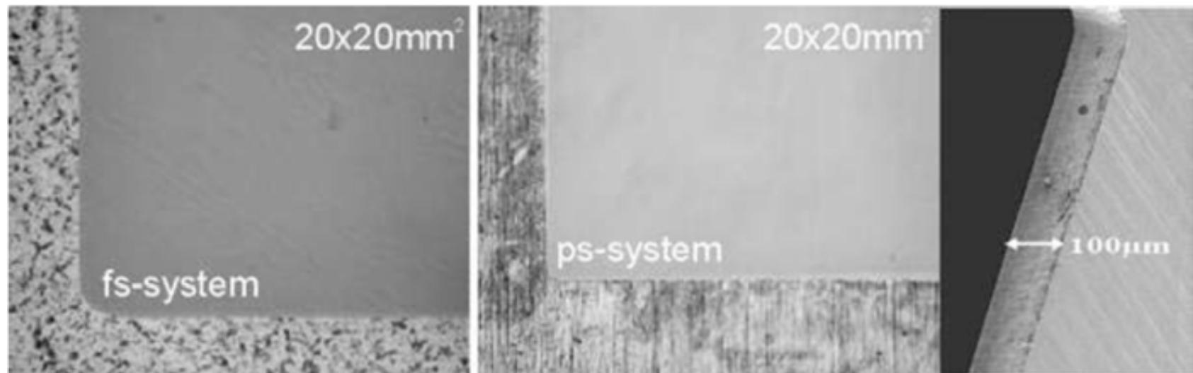
Cutting of 50  $\mu\text{m}$  steel sheet
