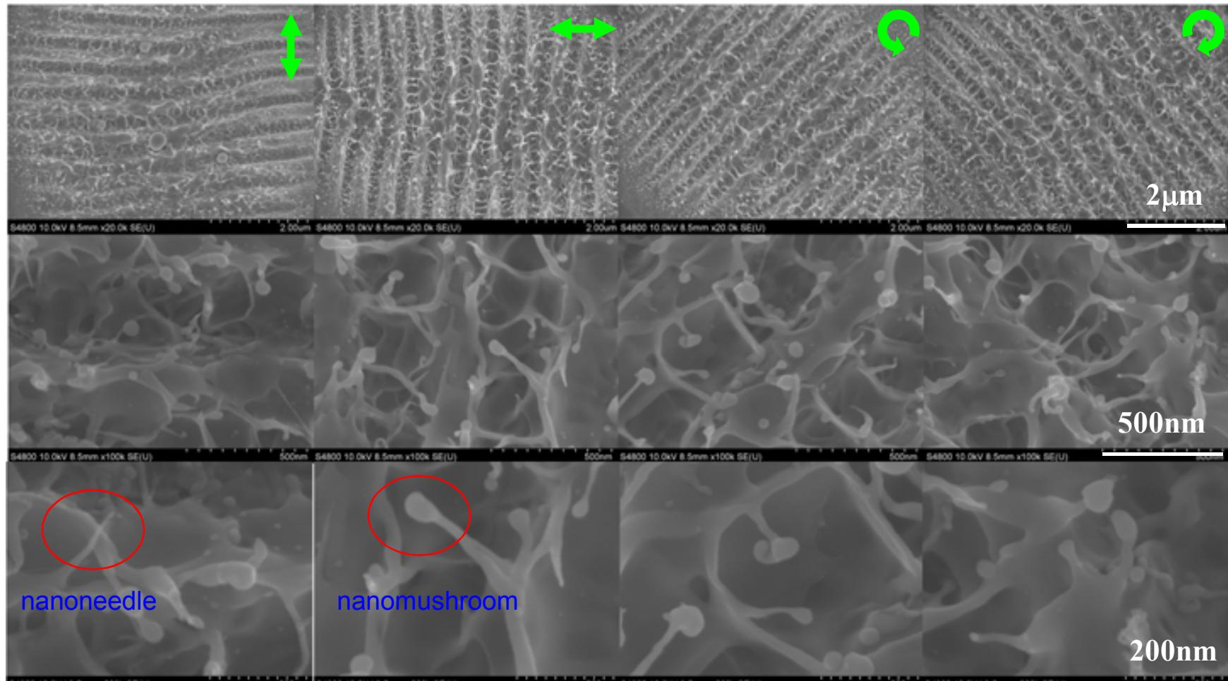
The nanospikes have a diameter ranging from 10 to 100 nm (at the neck of the mushroom-like spike) and up to 250 nm in length.
