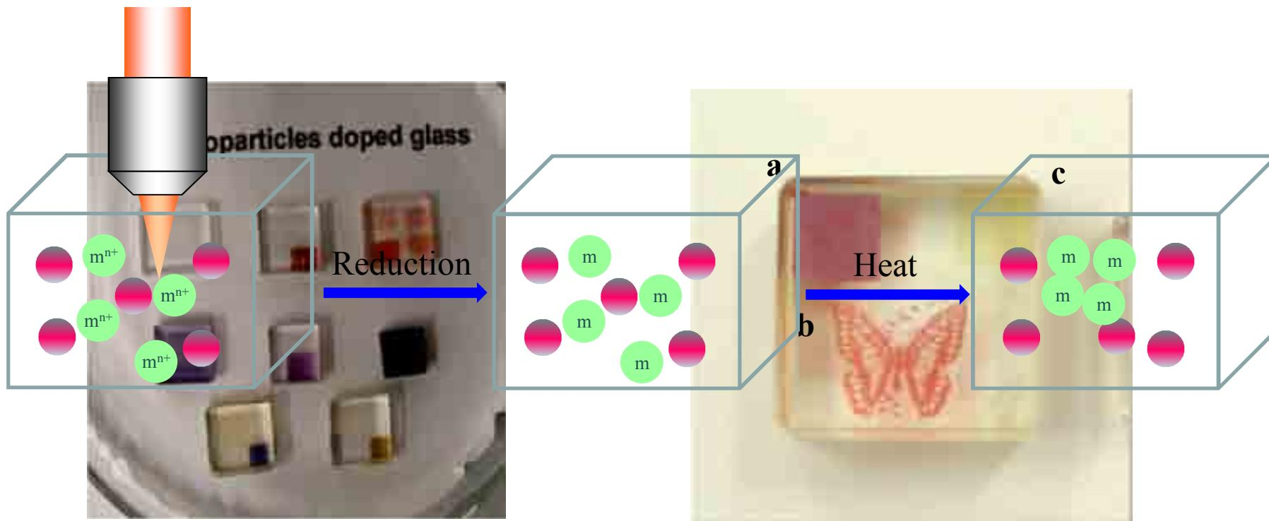
**Refractive index change in femtosecond laser irradiated Au<sup>3+</sup>-doped silicate glasses**
