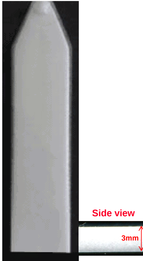
Mcell with mold temp. control Without GCP Mold temp. : 120°C
