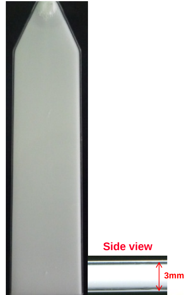
Mcell with GCP+mold temp.control GCP : 150 bar Holding time : 5s Dynamic mold temp. : 120°C
