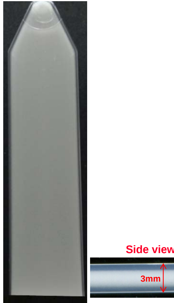
Mcell with GCP GCP : 150 bar Holding time : 5s Mold temp. : 40°C
