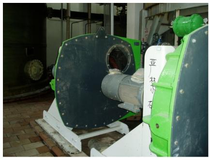
Hose pumps increase process yields by increasing thickened metal content & reducing maintenance costs
