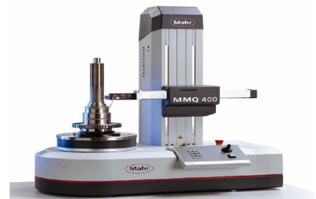
Roundness tester MAHR MMQ 400 To check the concentricity and roundness of the shaft
