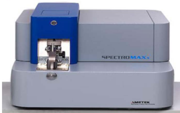
METALLOGRAPHIC LAB Spectro Photometer AMETEK SPECTROMAX F To check all material chemical composition
