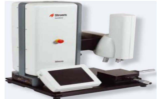
Microhardness STRUERS DURASCAN 20 To check the hardening depth
